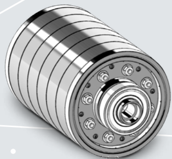
Assembled and balanced rotor - ready for installation
